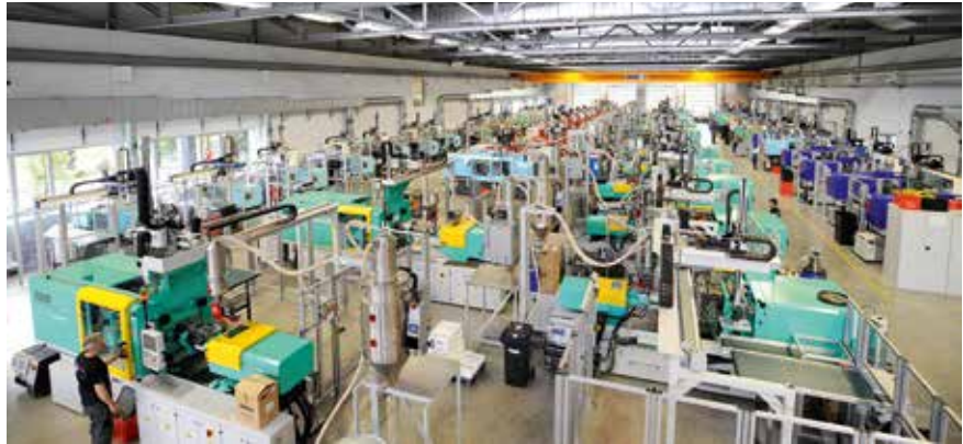
Fig. 3. Hörl specializes in the highly automated production of small and micro injection-molded parts. Thanks to the spot cooling solution from Linde, the company has increased the quality of its parts and reduced cycle times (© Hörl)
