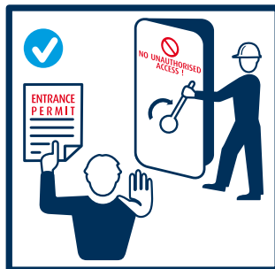
Permission to enter a confined space shall be given only after the issue of an entry permit.
