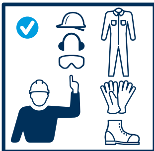
Proper clothes and personal protective equipment e.g. gloves and safety shoes must be worn.
