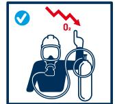
Breathing equipment must be used in situations where oxygen deficiency due to high CO<sub>2</sub> (>3%) content has to be expected.
