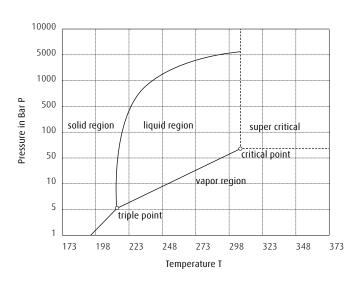
Triple point: T = 56.6 °C (216.55K) P = 5.18 bar abs Critical point: T = 31 °C (304.15K) P = 5.18 bar abs
