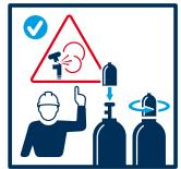
Cylinder valves must be protected against damage by screwing on cylinder caps.
