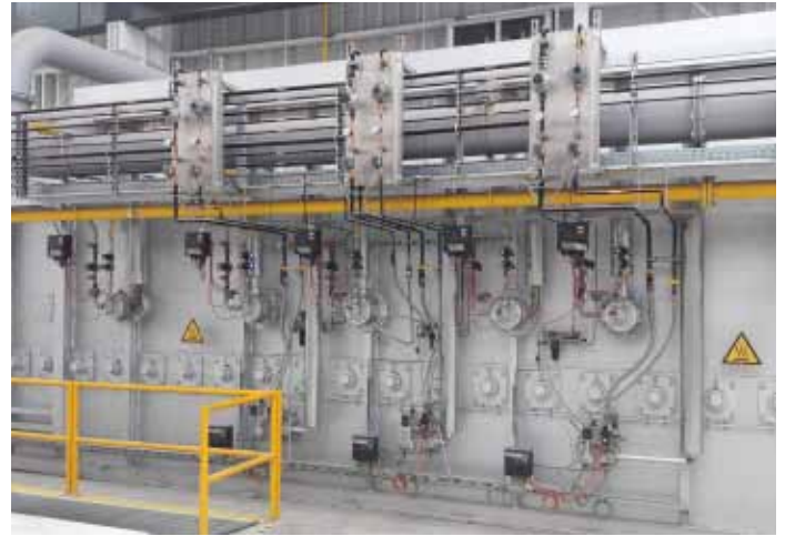
As an essential part of the installation, CARBOCAT® in-situ catalysts are used to produce high-quality endothermic gas.
