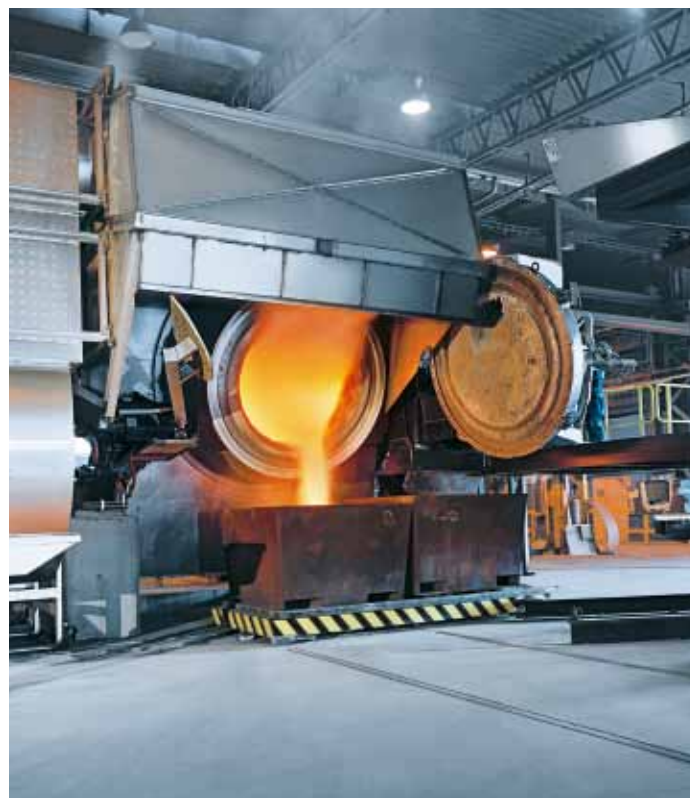
Stena Aluminium AB, Sweden, recycles scrap in two TRFs equipped with Linde's oxyfuel and WASTOX technology.
