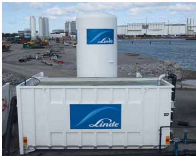
SOLVOCARB® neutralization basin in operation, complete with liquid CO 2 supply scheme
