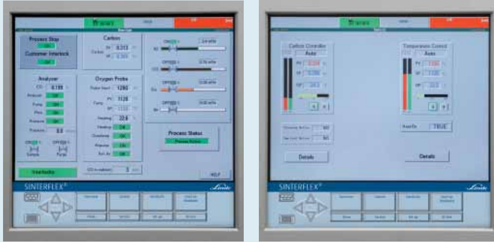
User-friendly customer interface for real-time monitoring and dynamic adjustment of furnace atmosphere
