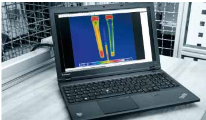
Direct comparison in practical trials with colour-coded temperature areas: When using carbon dioxide, the part cools down faster (right) than when using nitrogen (left). The trials showed equally high-quality results with a significant reduction in cycle times
