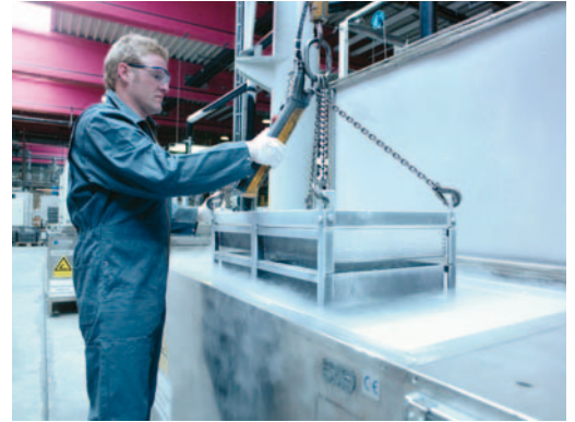
Sub-zero treatment of the charge after carburising to reduce retained austenite.
