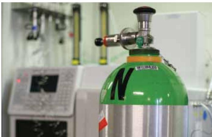
HiQ calibration gas mixture cylinder for gas chromatograph calibration.
