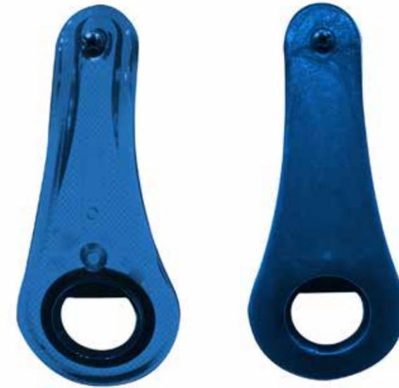
Bottle openers produced using solid injection moulding (left) and foam injection moulding (right)
